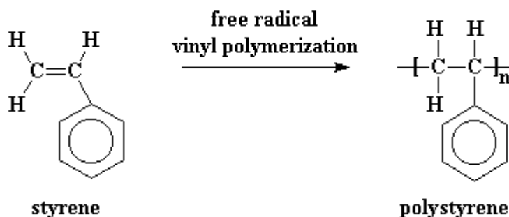
5 POLYMERIZATION OF STYRENE INTO POLYSTYRENE (“POLYSTYRENE,” N.D.)
