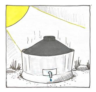
Our solution arrives in the camp. It is a solar powered water desalination and purification device. If regularly filled with unclean sea water and left out in the sun, each device will provide the refugees with 5 litres of potable water every day.
