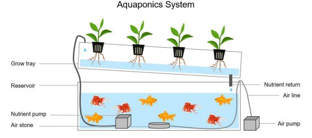
Aquaponics is the method of cultivating plants as well as growing aquatic organisms. It basically puts a hydroponic system and an aquaculture together, using the fish waste as a fertilizer for the plants. The water from the fish tank goes through a biofilter, in which bacteria convert the fish waste into useful nutrient solution. Those solutions will then go to the roots of the plants and the roots will take the water and nutrients.
