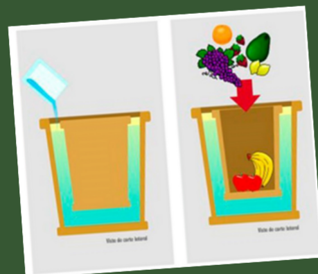
Zeerpot: cheap, no electricity refrigerator
