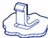
L-Shaped Snap Joints
