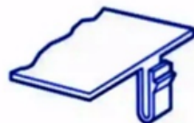
U-Shaped Snap Joints
